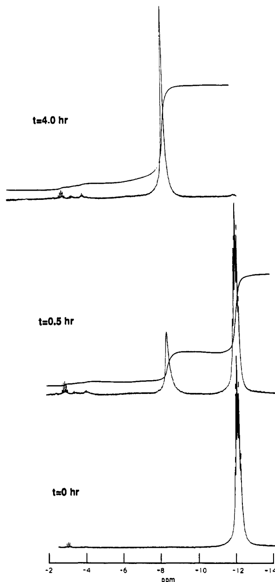
Figure 1. 31 P NMR spectra obtained during 125 °C polymerization in diglyme ([M] 0 = 1.5 M; [I] 0 = 0.015 M).
